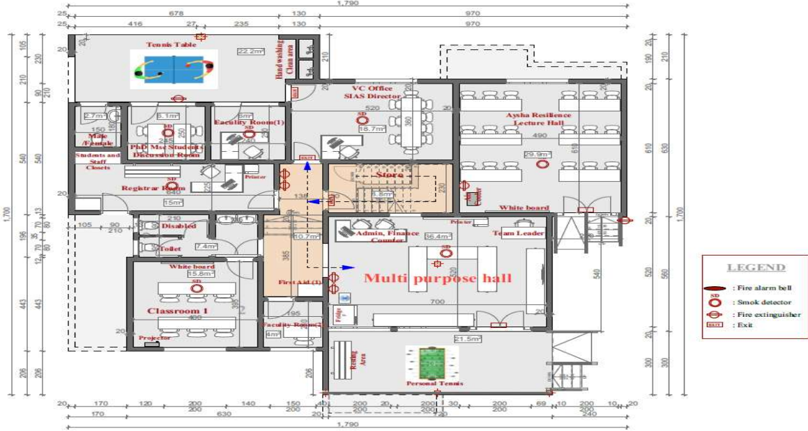
Figure (1b) SIAS Building Drawings showing Distribution of Fire Detectors and Fire Escape route in case of Evacuation for (First Floor).
